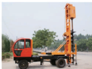
Spiral pile driver
